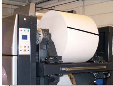
Core acceleration is standard on all MP models. This allows easy straight-across splice preparation.
