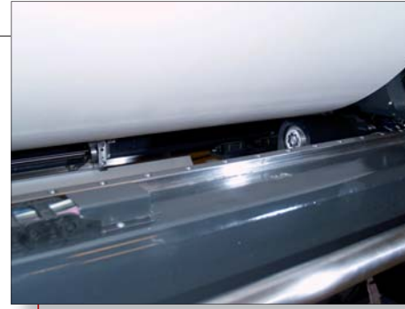
Unique mechanical transmission with spline shafts for high design modularity between 2-Quadrant and 4-Quadrant drive systems
